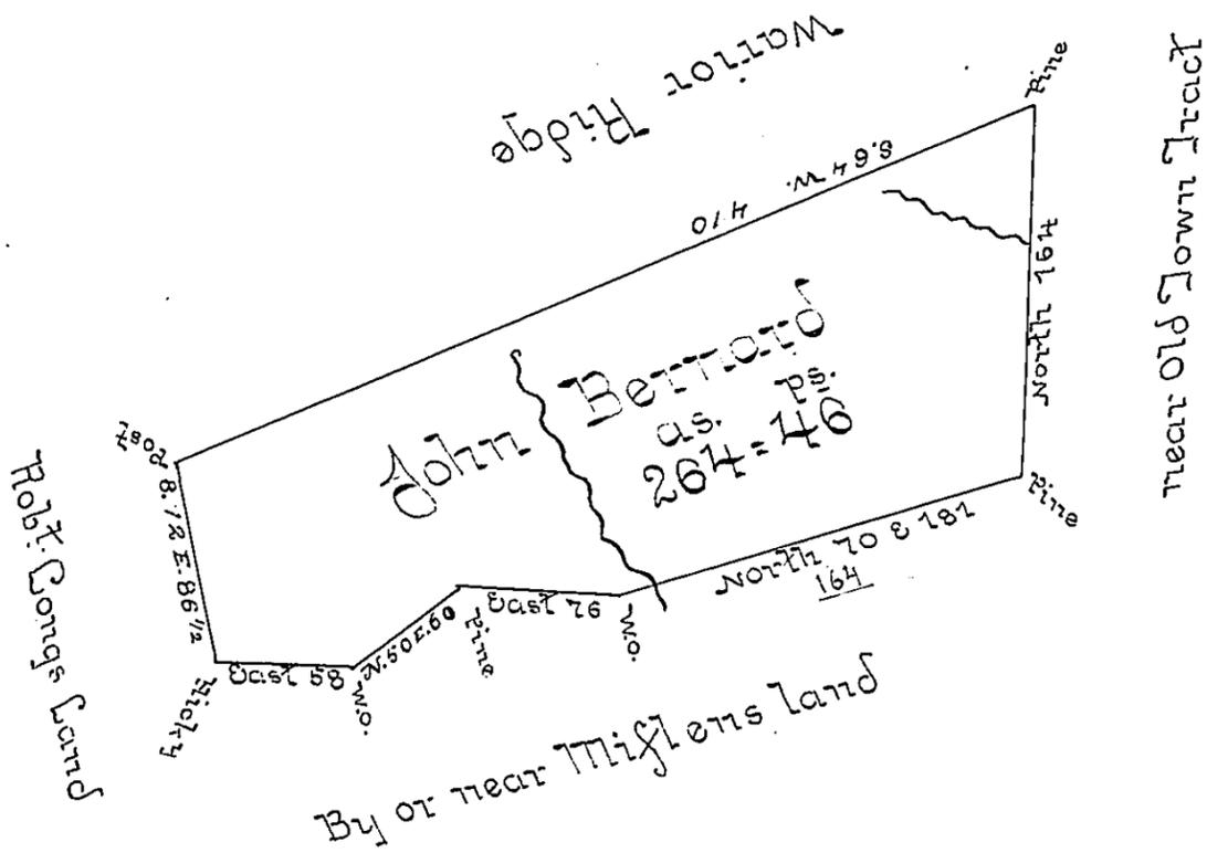
Situate near & below Old Town Tract on the Waters of Standing Stone Creek about Two Miles & a half above the Warm Springs in Barre Township in the County of Bedford containing 264<sup>acs</sup>. 46<sup>ps</sup>. and the Usual Allowance of Six per Cent for Roads Surveyed the 3<sup>d</sup> day of June 1785 in pursuance of a Warrant Dated the 2<sup>d</sup> Day of November 1784.
